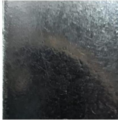
Fig.2 Photograph of developed Galvanized coating
