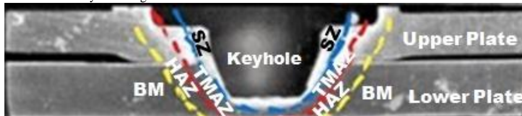
Fig.2 Typical schematic of microstructural zones in FSSW
