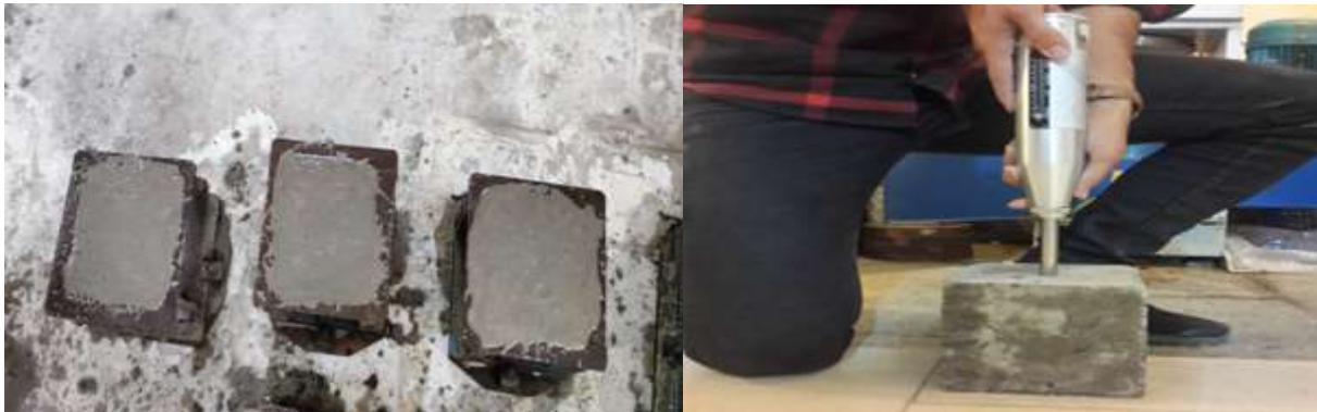
Fig. 1. (a) JFRC Cube moulds (b) Rebound hammer testing in laboratory
